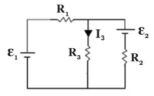
Determine the current (  $\mathbf{I_3}$  ) through resistor  $\mathbf{R_{3.}}$
