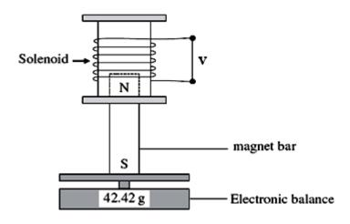
a- Does the reading of the electronic balance decrease or increase after the solenoid is lifted straight up? Explain. (2 marks)
