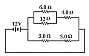
The current in the (4.0  $\Omega$ ) resistor is:
